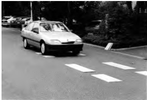
Fig. 24.64. Driving experiment with wooden plates to excite the vertical dynamics
