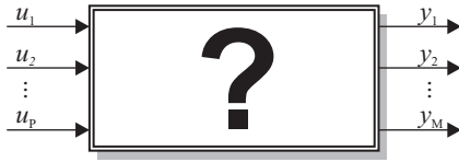
Fig. 20.1. System with P inputs and M outputs, which has to be approximated by an artificial neural network (ANN)
