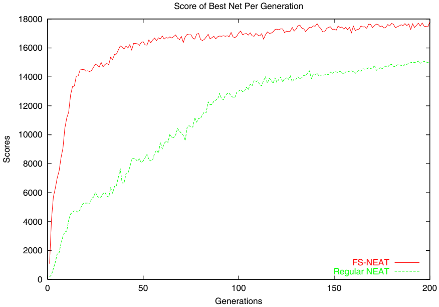
Fig. 6.4 A comparison of the performance of regular NEAT and FS-NEAT in the RARS domain with 162 available inputs, 80 of which are irrelevant to the task. Each line in the graph represents the score received by the best network from each generation, averaged over all 10 runs. By learning appropriate feature sets, FS-NEAT learns significantly better networks and learns them faster than regular NEAT.
