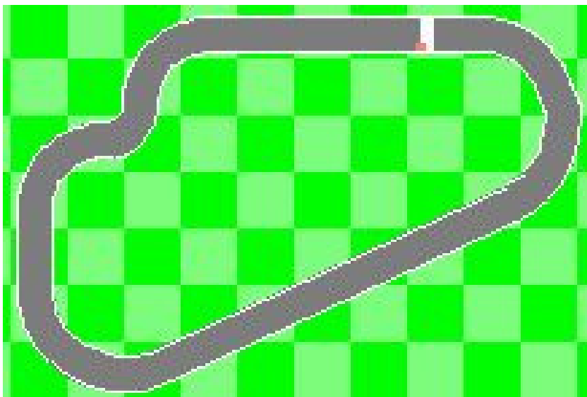
Fig. 6.3 The “clkwis” track used in the FS-NEAT experiments. It captures a wide range of driving challenges (i.e. straight sections, turns, and an S-shaped curve).
