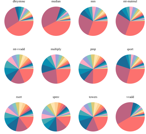
Fig. 4: The importance proportions for each architectural parameter to the benchmark programs. Each segment in the pie chart represents the proportion of sensitivity of benchmark performance to microarchitecture parameters.
