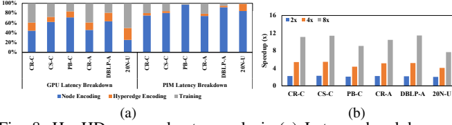
Fig. 8: HygHD on accelerator analysis (a) Latency breakdown of HygHD on GPU and PIM (b) Scalability of HygHD
